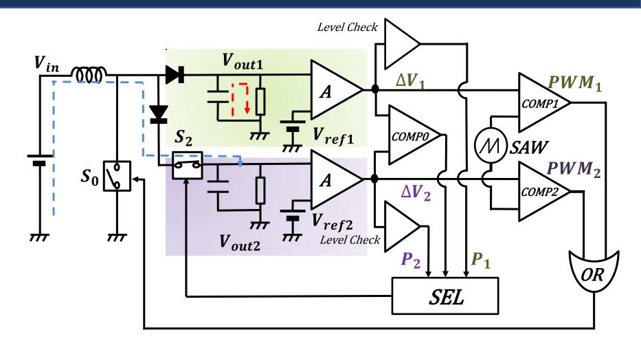
In one period: 3. Inductor uncharge,  $S_0$  keep OFF.  $\Delta V_1 > 0, \Delta V_2 < 0, P_1$  Low,  $S_2$  turn ON,  $P_2$  keep High
