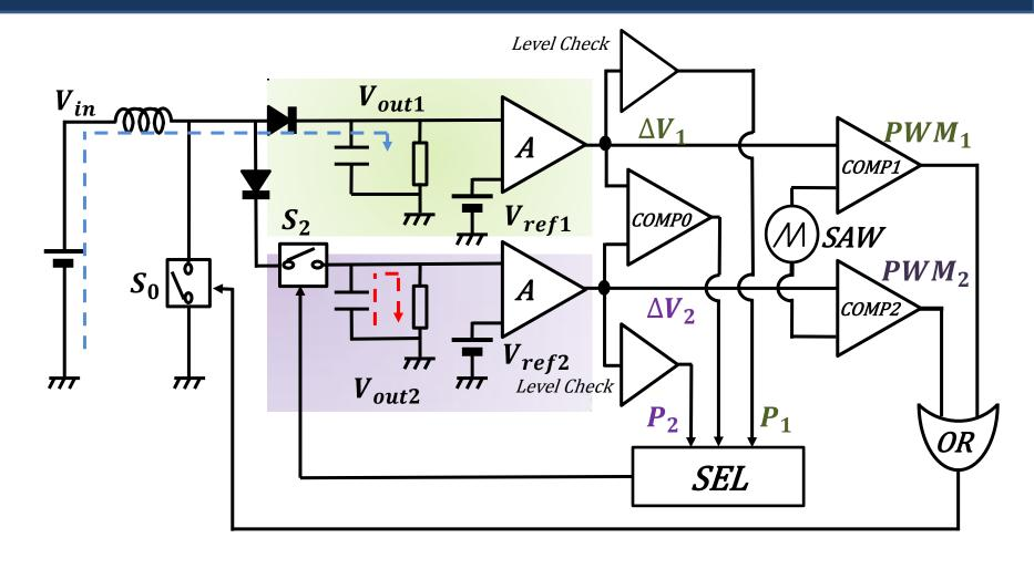
In one period: 2. Inductor uncharge,  $S_0$  turn OFF. If  $\Delta V_1 < \Delta V_2 < 0$ ,  $S_2$  OFF,  $P_1$  and  $P_2$  both are High.
